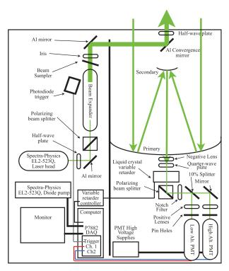
FIG. 4. Schematic layout of optics and main components of CAPABL. Lidar transmits a single linear polarization and detects linear polarizations parallel, perpendicular, and at 45° to the transmitted polarization.
