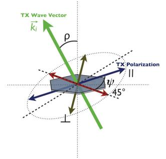
FIG. 2. Illustration of the polarization terms in reference to the lidar beam and horizontal scatterers. Lidar tilt angle ( $\rho$ , 11° for CAPABL) is measured relative to zenith (vertical axis), and the polarization angle  $\psi$  is measured relative to the linear polarization that lies in the horizontal plane (plane perpendicular to the **k** of the transmitted light). Dashed oval represents the plane perpendicular to the vector of the transmitted beam.
