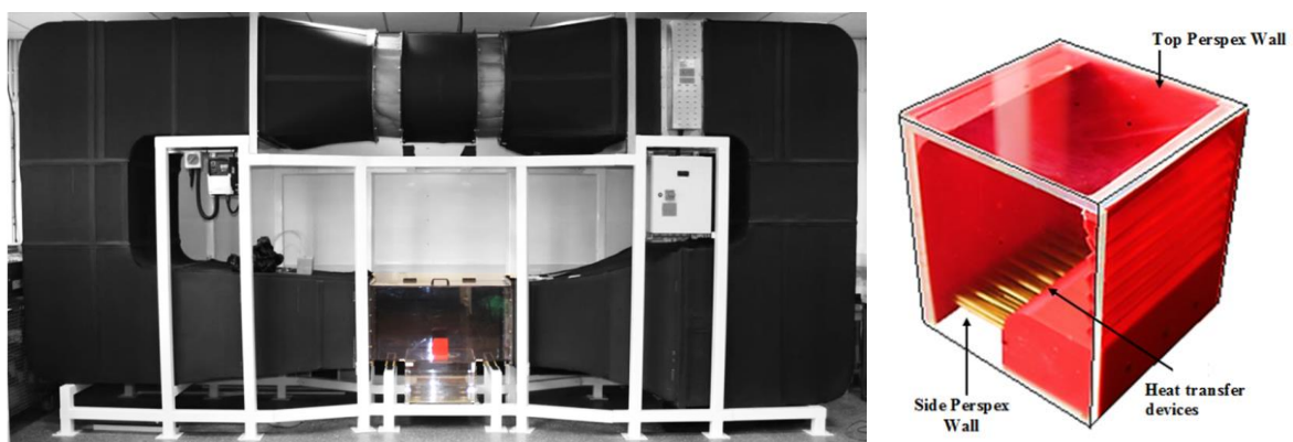
Figure 5: Low-speed wind tunnel (left) 3D printed model (right) [24, 25].
