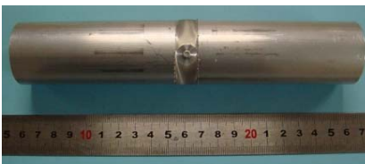
Figure 2. Al 6082-T6 FS welded tubular specimen.
