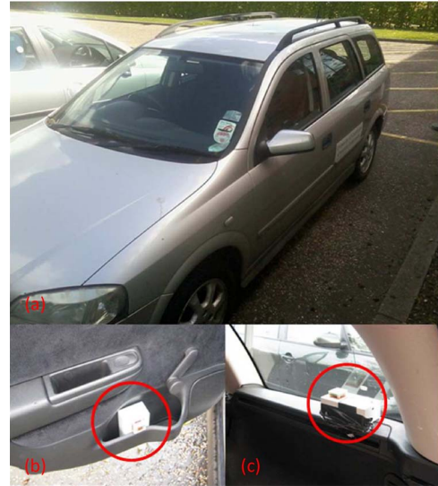
Fig. 4. (a) Car; (b) transmitting node located in the passenger side rear door; (c) receiving node located in the boot on the driver side.
