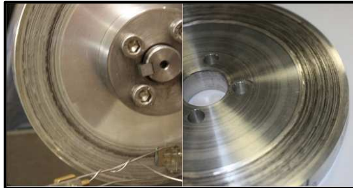
Figure 4: Uncoated aluminium alloy rotor after test showing badly degraded rubbing surface
