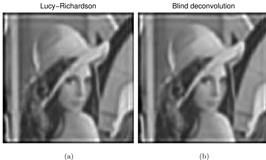
Fig. 4. Deblurred images of the image in Figure 2(b) obtained by (a) the Lucy-Richardson algorithm and (b) blind image deconvolution, for Example 1.
