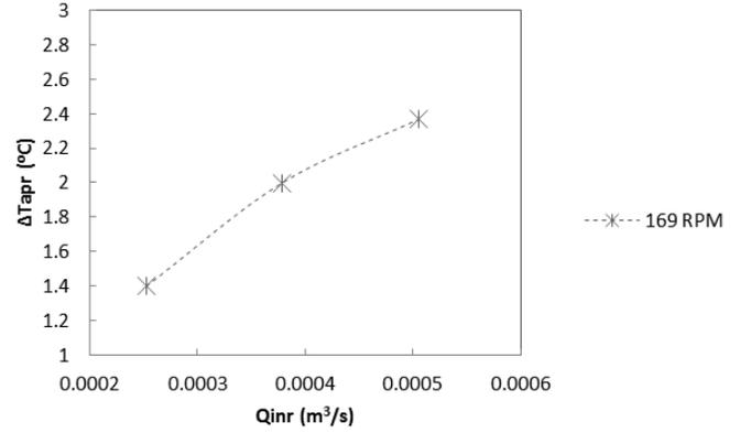
Fig. 3. The variation of  $\Delta T_{apr}$  with flow rate  $Q_{inr}$ , dry cooler fan spins at 169 rpm.
