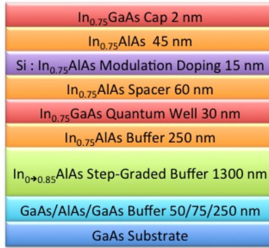
Figure 1: Schematic layer structure of In 0.75 Ga 0.25 As/In 0.75 Al 0.25 As Quantum Wells
