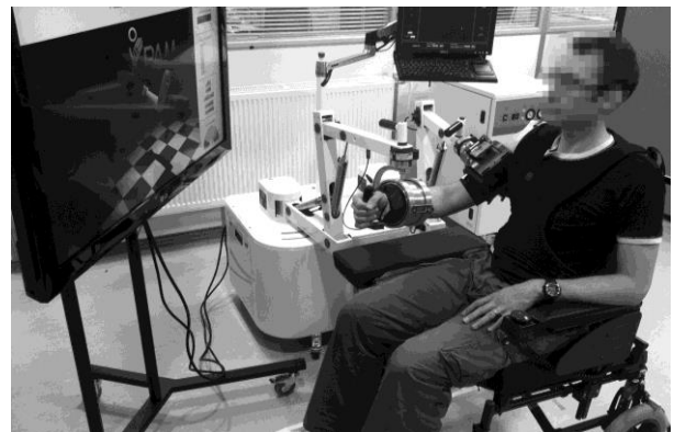
Figure 1. The iPAM MkII Robotic Rehabilitation System
