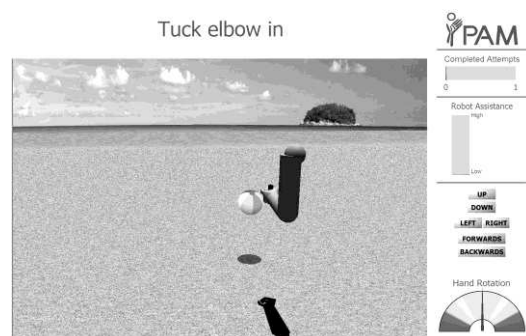
Figure 2. Patient Interface screen appear on a large display in front of patient during exercise and displays human arm model and virtual targets.
