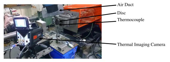
Figure 2: Full Scale Brake Dynamometer Test Rig.
