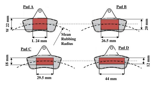
Figure 1: Brake Pads with Different Aspect Ratios (edited [9]).
