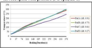
(f) High speed-Med pressure (925 rpm, 2.5 b)
