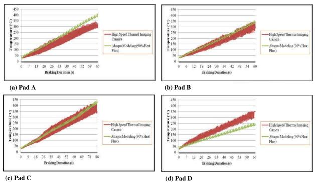
Figure 6: Comparison of simulation and experimental data at high speed and high pressure (925 rpm/4.5 Bar).
