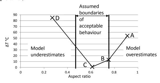
Figure 7: Performance of validated model as a function of aspect ratio.
