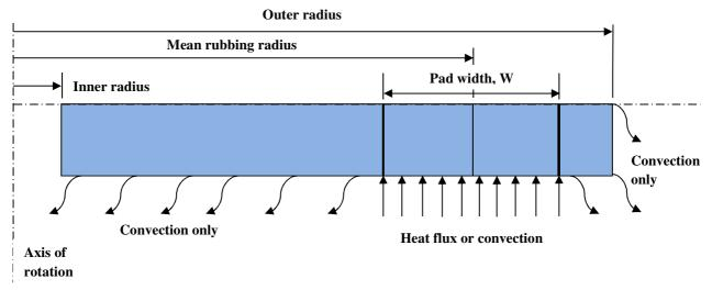
Figure 4 Outline of finite element model.
