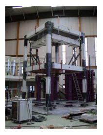
Figure 10: Retrofitted frame on AZALEE shaking table
