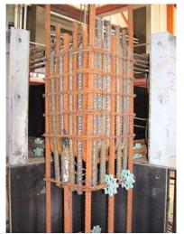
Figure 5: Reinforcement of a 1<sup>st</sup> level node
