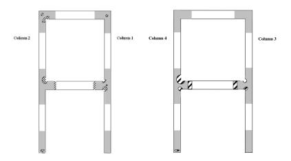
Figure 16: Debonded areas of FRP after 0,5 g seismic test – (Front-back elevations)
