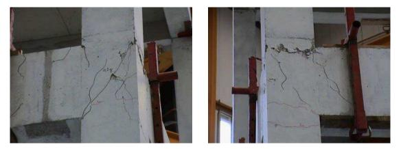
Figure 14: Views of the cracks and the first slab level of the mockup after the first series of tests without strengthening
