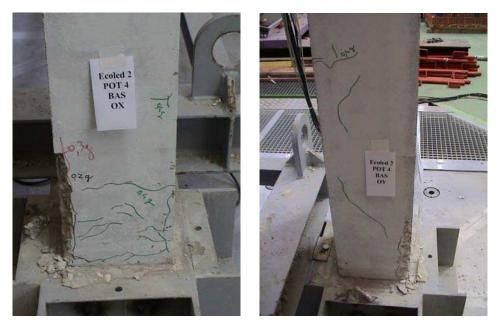
Figure 13: Views of the cracks and the bottom of the columns of the mockup after the first series of tests without strengthening
