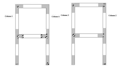
Figure 17: Debonded areas of FRP after 0,5 g seismic test – (Side elevations)
