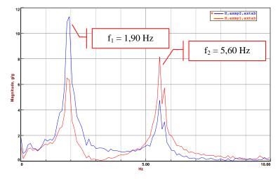
Figure 18: Natural frequency measurements -Bare frame before seismic tests
