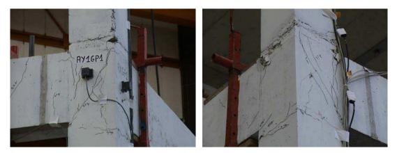
Figure 15: Views of the cracks at the first slab level of the mockup after the first series of tests without strengthening
