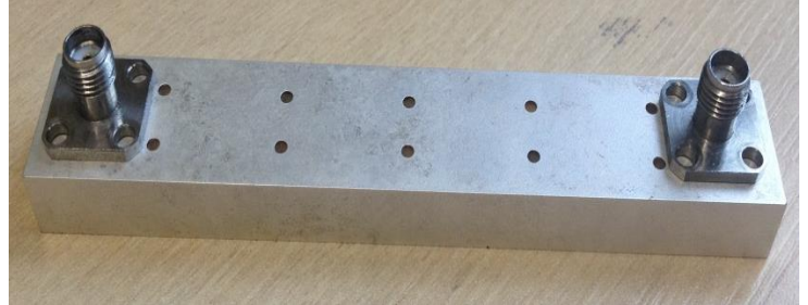
Fig. 6. Fabricated six pole chebyshev ceramic waveguide filter
