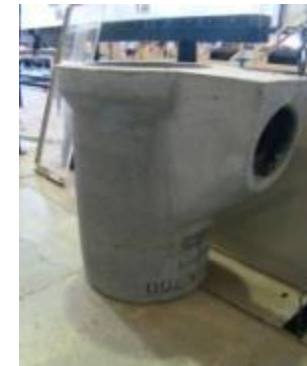
Modern trapped UK gully (375mm diameter, 750mm depth) with 150mm diameter outlet
