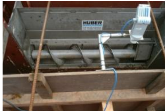
CSO screen in full scale test rig
