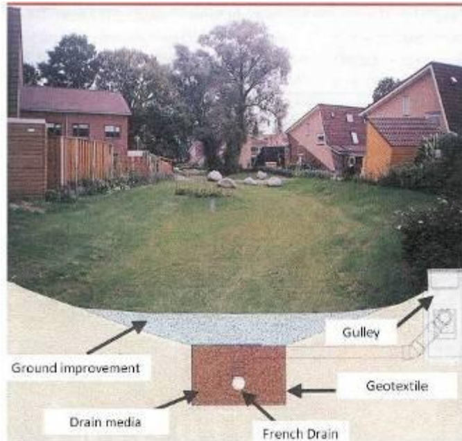
Cross section through a Wadi (UWC)
