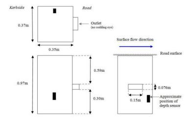
Figure A4.3: Details of Gulley and location of sensor, Monitor B
