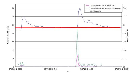
Figure A4.6: Depth and Discharge curves for Gulley A on 7<sup>th</sup> July 2012 (Calculated discharge based on impermeable area)
