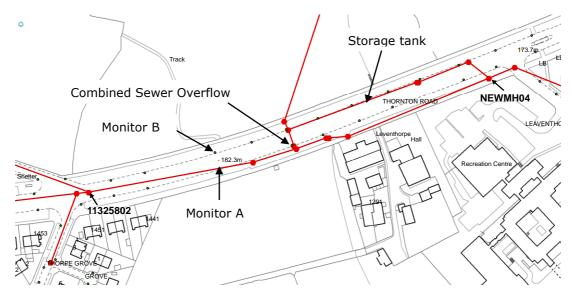
Figure A3.7: The combined sewer system in Thornton Road
