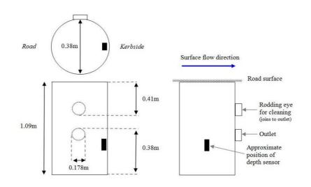
Figure A4.2: Details of Gulley and location of sensor, Monitor A
