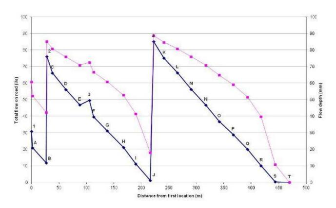
Figure A5.2: Depth and flow rate along highway
