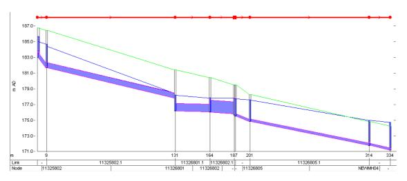
Figure A3.8: Hydraulic grade line for a 30 minute event with an annual probability of 1%.
