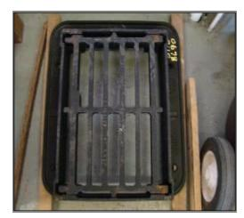
Figure A2.7: Grate with 400mm x 432mm clear opening (HA102 Reference – R)
