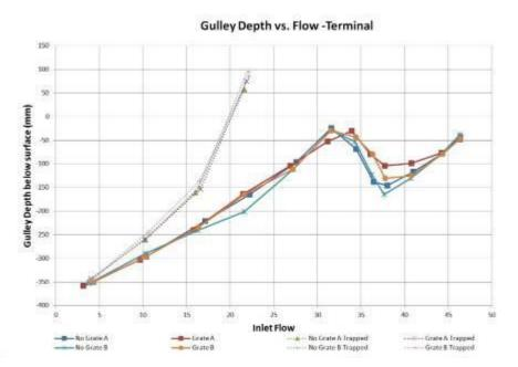
Figure A2.10: Depth discharge relationship for the gulley with different grates and with and without the rodding eye plug in place
