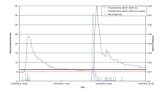
Figure A4.9: Depth and Discharge curves for Gulley B on 7<sup>th</sup> July 2012 (Calculated discharge based on impermeable and saturated permeable areas)
