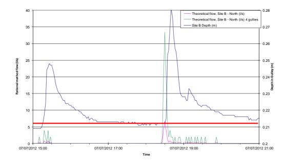
Figure A4.8: Depth and Discharge curves for Gulley B on 7<sup>th</sup> July 2012 (Calculated discharge based on impermeable area)
