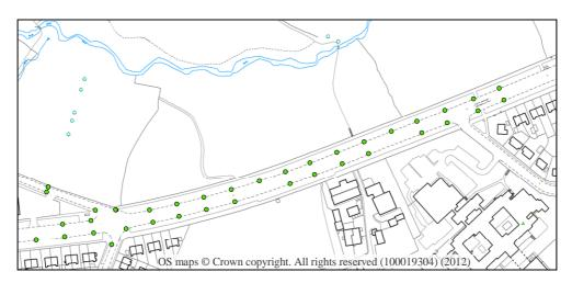
Figure A3.1: Monitoring and case study site, surveyed gully locations shown as green circles
