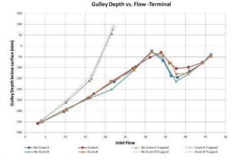
Figure 4.1.1: Depth discharge relationship for the gulley with different grates and with and without the rodding eye plug in place
