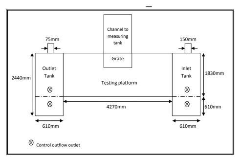
Figure A2.2: Dimensions of the laboratory rig
