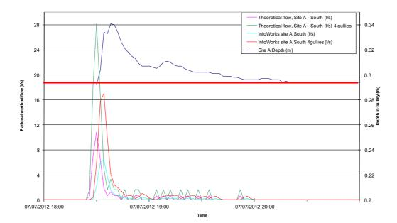
Figure A4.10 application of fixed PR runoff model and Wallingford routing to calculation of flow rates for Gulley A
