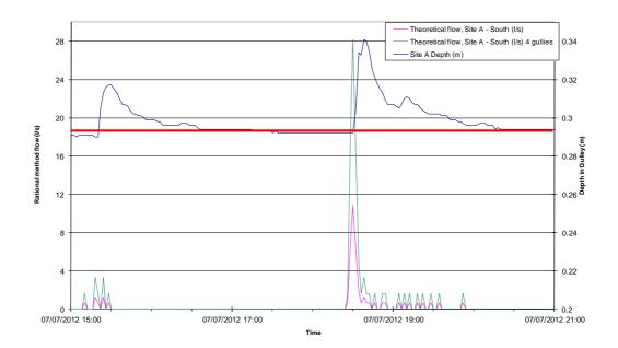
Figure A4.7: Depth and Discharge curves for Gulley A on 7<sup>th</sup> July 2012 (Calculated discharge based on impermeable and saturated permeable areas)
