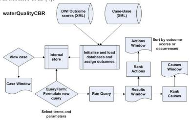
Figure 1. WaterQualityCBR software system main operations (from [4])
