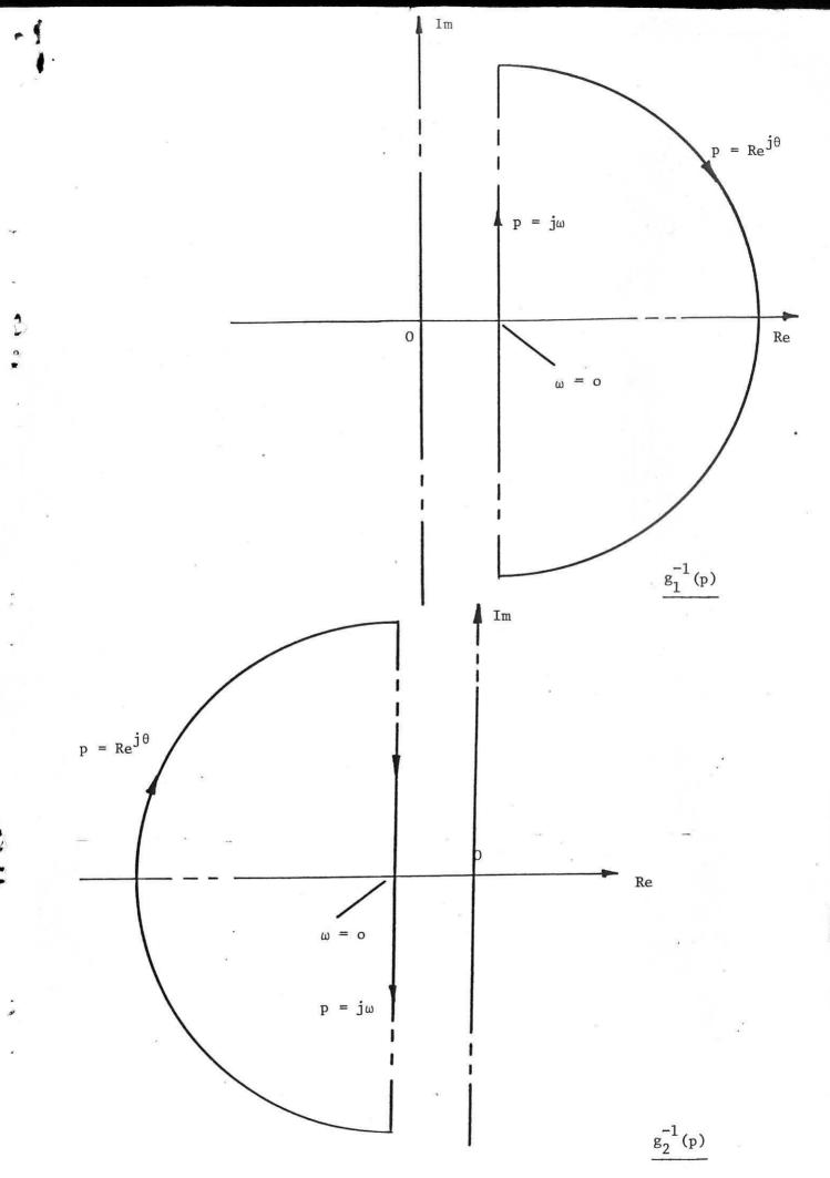
Fig. 5 Basic shapes of inverse Nyquist loci for tray-column
