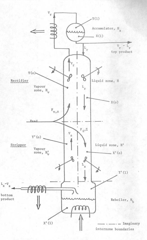
Fig. 1 Zoning and main variables in packed-column
