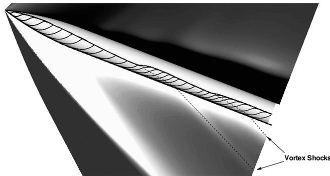
**b) Predicted symmetry plane density gradient ( $\nabla\rho$ ) and surface skin friction lines**
