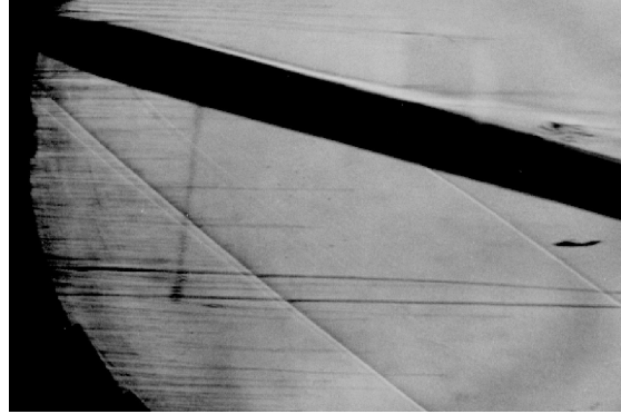
Figure 1: Schlieren Picture for Supersonic Flow around an Ogive Cylinder at M=1.8 , \alpha=14^\circ , Re/D=6.6 \times 10^5
