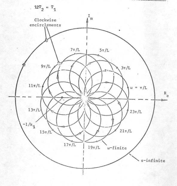
Fig. 2 Inverse Nyquist Diagram for Rolling Process
