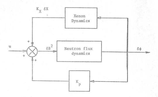
Fig. 5.5. Inherent feedback loops in long-term reactor spatial dynamics
