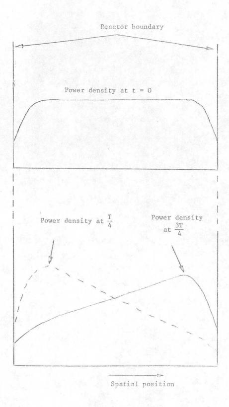
Fig. 5.1. Power density oscillation of period T in a one-dimensional nuclear reactor
