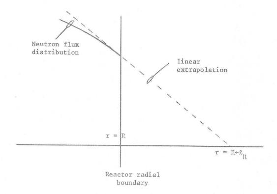
Fig. 5.3. Boundary condition construction
