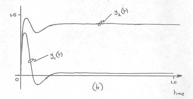
Fig. (a) Response to a unit step demand in ontput one.
