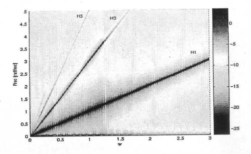
Figure 7. Response Spectrum Map for Duffing Equation (10)
