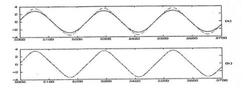
Figure 5 (a) First order output response, and (b) up to the third order response Solid—synthesized output from the GFRF's of eqn (9); Dashed-- original output from (4)
