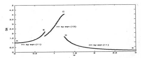
Figure 11. First order frequency domain response function for the Duffing oscillator (10)
