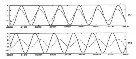
Figure 10 (a) First order output response, and (b) up to the third order response Solid—synthesized output by GFRF's from (10); Dashed—simulated original output from (10)
