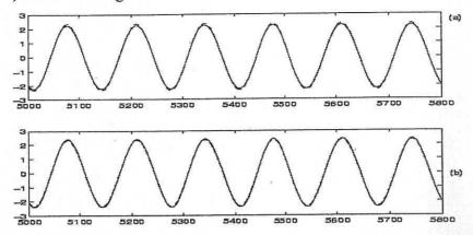
Figure 9 (a) First order output response, and (b) up to the third order response Solid—synthesized output by GFRF's from (12); Dashed-simulated original output from (10)
