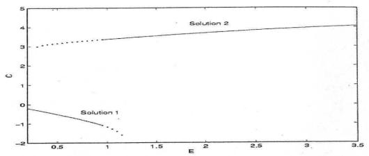
Figure 3. Response amplitude curves using the harmonic balance method
