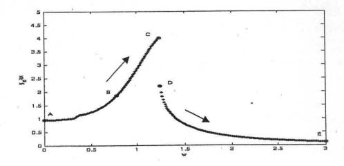
Figure 6. Resonance response curve for Duffing Equation (10)
