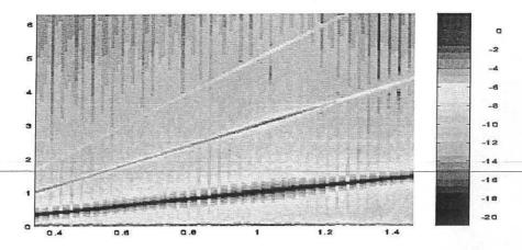
Figure 1. Response Spectrum Map of Duffing Oscillator (6)
