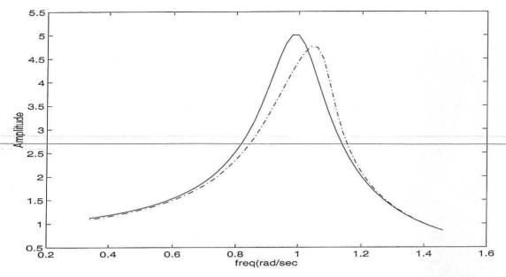
Figure 2.  $H_1$  from original Duffing equation (6) –Solid and  $H_1$  from NX modelling—Dot Dashed
