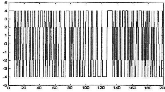
Figure 2 The PRBS used as the system input to identify the linear dynamics for Example 1
