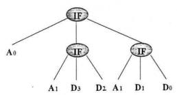
**Fig. 6.** Hierarchical encoding of the 6-multiplexer function.
