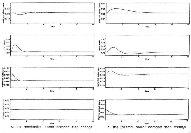
Fig. 9 : The turbine response with two PI regulators for pass-out steam pressure and rotor speed
