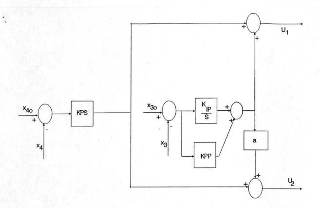
Fig. 6: The regulator with a PI for paa-out steam pressure and a P for rotor speed
