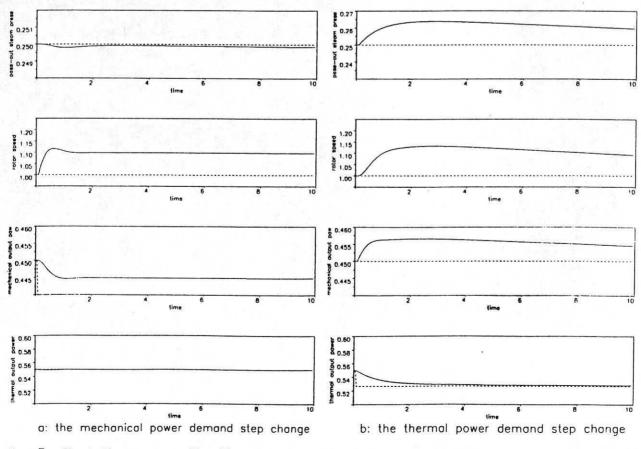
Fig. 7 : The turbine response with a PI regulator for pass-out steam pressure and a P regulator for rotor speed
