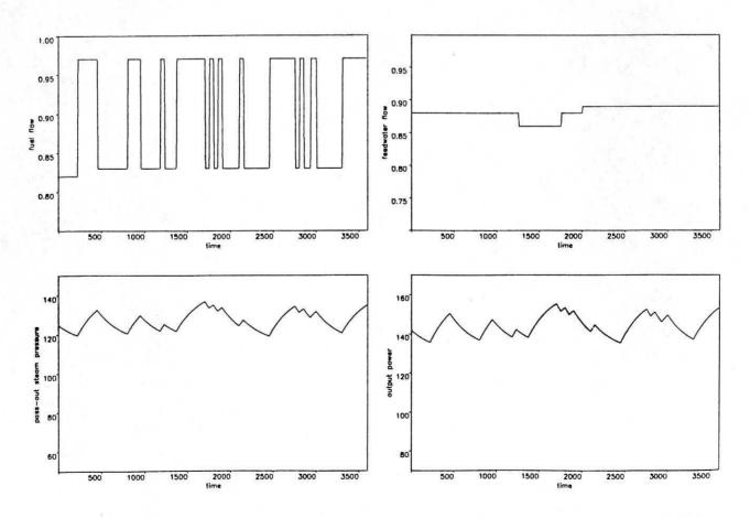
fig. 5 : Simulation of new drum-boiler model
