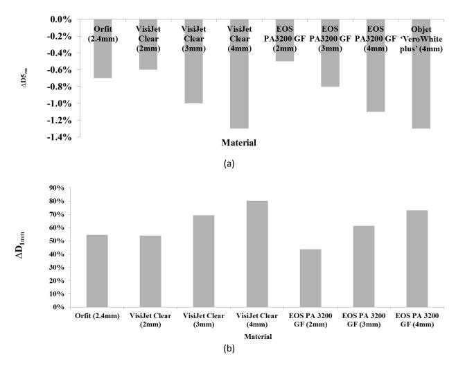
Fig 2: (a) The change in dose at 5 cm depth,  $\Delta D_{5cm}$  for the Orfit thermoplastic mask in comparison to three different 3D printer materials. (b) The change in dose at 1mm depth for the Orfit thermoplastic mask in comparison to three different 3D printer materials.
