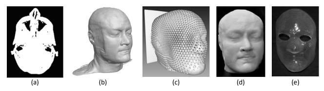
Fig 1: Constructing the masks from MRI data. (a) Image of a slice of the MRI data which has been segmented using Osirix, (b) 3D computer model of the head derived from the segmented MRI data set, (c) Edited 'negative' shell (holes were subsequently formed in the shell to demonstrate the possibility of further reducing material cost), (d) 3D print of the model of the head and (e) 3D print of an example 'negative' shell.
