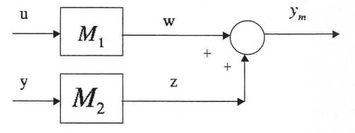
Figure 2. Implementation of independent model for open-loop simulation
