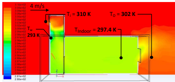
Figure 17 Temperature distributions within the test room with external wind speeds of 4 m/s (Evaporative cooling)
