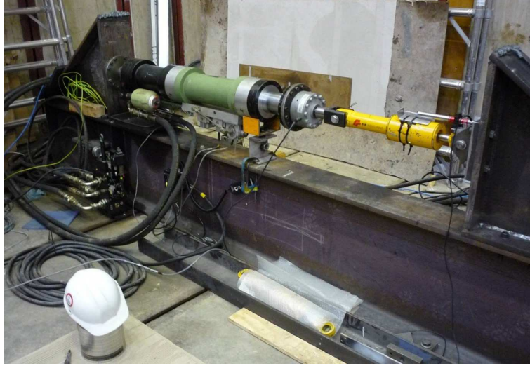
Figure 14: Experimental rig set-up of substructured model.
