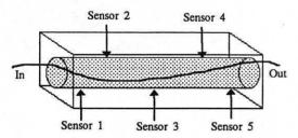
Figure 4 The extended "circle-in-the-square" task requires a system to identify whether a particle is travelling inside or outside a tube residing in a rectangular box.
