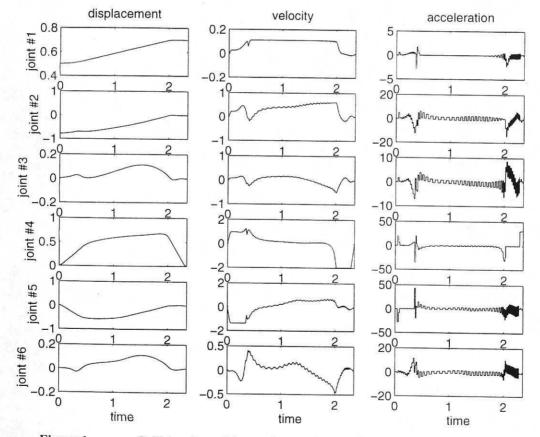
**Figure 1.** Collision-free minimum time motion for  $\mathbb{O} \rightarrow \mathbb{O}$ .
