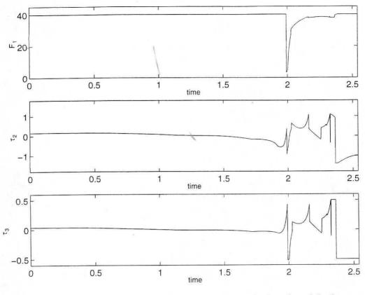
**Figure 7.** Profiles of the Force/ Torques for time-optimal motion of the first three joints of the RTX robot
