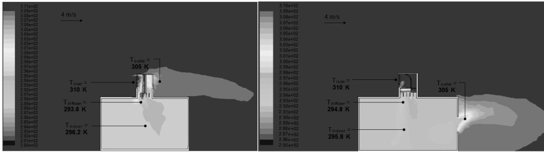
Figure 8: Temperature distributions inside the test room with a commercial wind tower incorporating the vertical HTD arrangement (a) and horizontal HTD arrangement (b).
