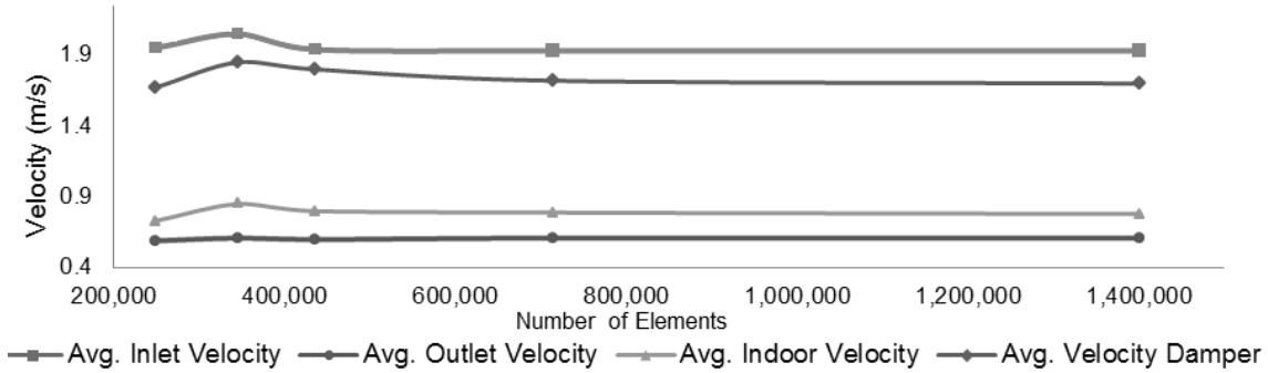
*Figure 5: Comparison of solutions from various grid adaptation methods. The variables are the average velocity at the inlet and outlet of the wind towers and interior of the test room*
