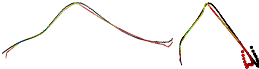
Fig. 8. Comparison of the real (black) and virtual (different colours) Terumo angled guidewires in the silicon rubber phantom. The insertion point is on the left and the tips are on the right. The virtual wire particles are blue when there is very good agreement (< 0.5mm), green for good agreement (> 0.5mm, < 1mm), yellow for an intermediate agreement (< 1mm, > 2mm), orange for a poor agreement (> 2mm, < 3mm) and red for a very poor agreement (> 3mm).
