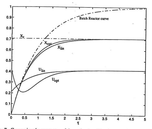
Fig. 7. Comparing the responses of the optimal and linarly controlled process for equal minimum flow conditions.
