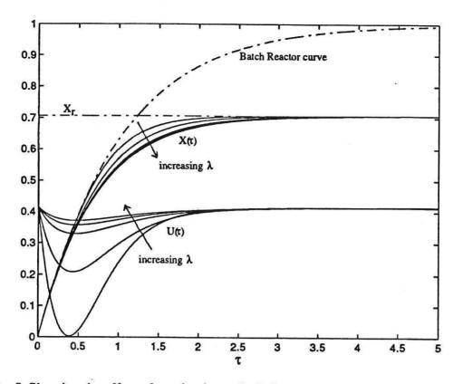
Fig. 5. Showing the effect of varying input deviation cost weighting on the optimally controlled process response.
