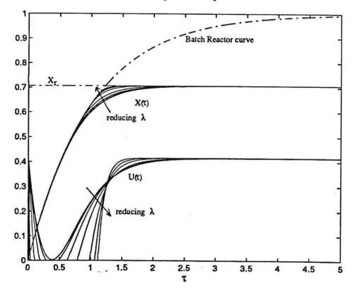
Fig. 6. Showing the effect of the non-negative flow constraint on the optimally controlled process with low input cost weighting.
