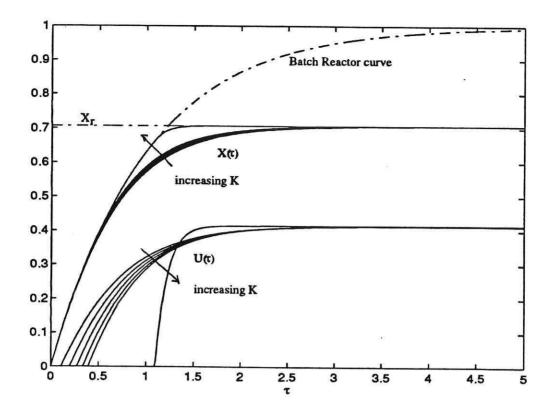
Fig. 3. Higher gain linear control, showing the effect of the non-negative flow constraint.
