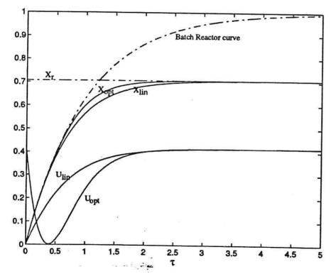
Fig. 8. Comparing the responses of the optimal and linearly controlled process for the maximum possible unconstrained input excursion.
