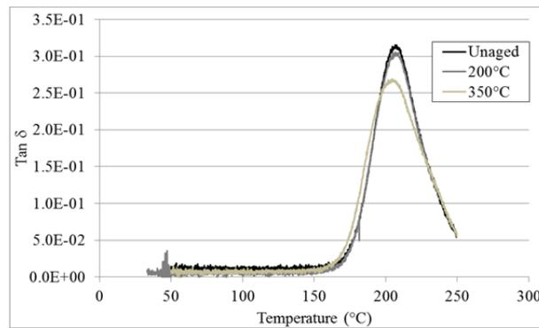
**Figure 2.** Results of the damping coefficients obtained in DMA tests (3-point bending configuration) for the three considered conditions, unaged, 200°C and 350°C.
