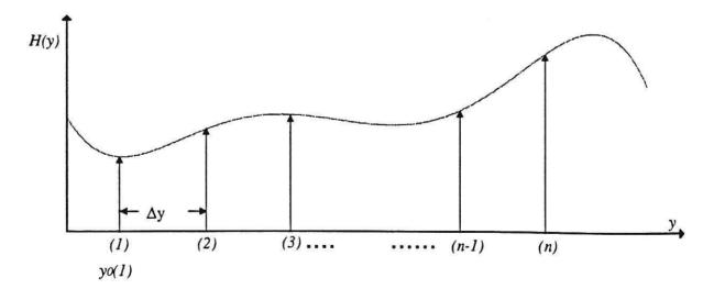
Fig. 3. The single scan solution uses n sampled values from a single scan to track a field of order n.
