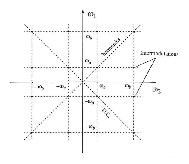
Fig.2 Input frequency domain(for two-tone input).
