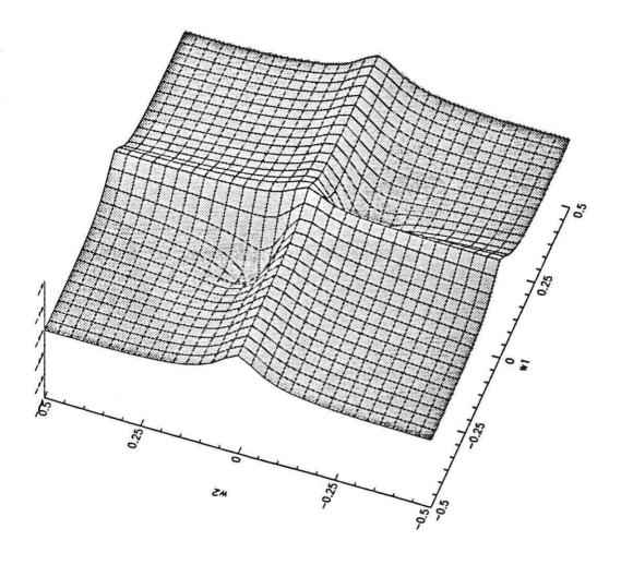
Fig.9 The magnitude of  $H_1(j\omega_1) + H_1(j\omega_2)$ .
