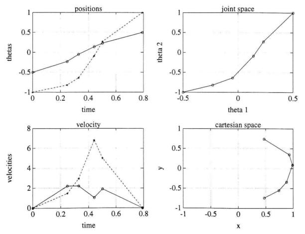
Figure 2: Optimum trajectory evolved after 5000 generations with 100 individuals in each generation; Joint one (-----) and joint two (----) in a 10x10 grid space.
