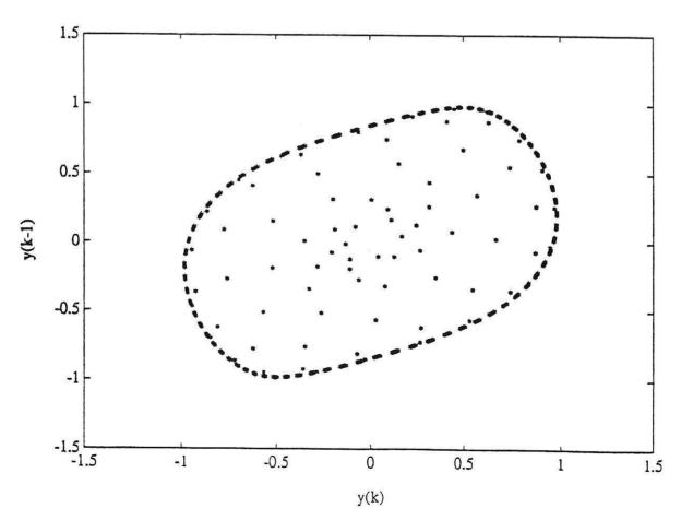
Figure 4.5 Limit cycle from the identified model with initial condition:  $\hat{y}(-1)=\hat{y}(0)=0.1$
