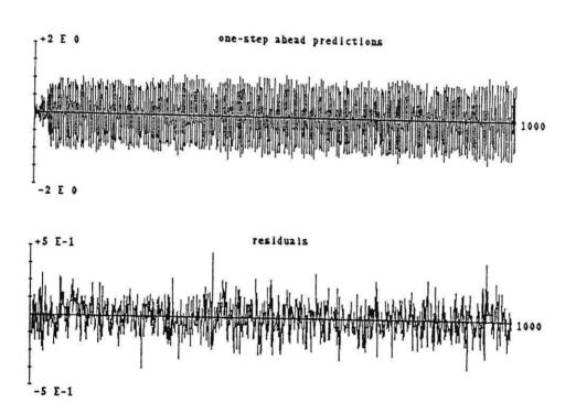
Figure 4.2 One step ahead predictions & residuals for the exponential time series approximation
