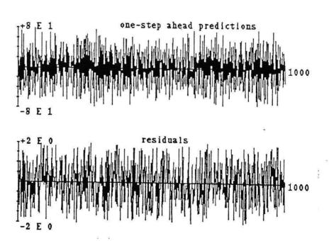
Figure 3.2 One step ahead predictions & residuals for the identified Morison's equation
