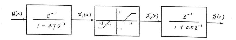
Figure 5.1 Dynamic system with dead zone & saturation
