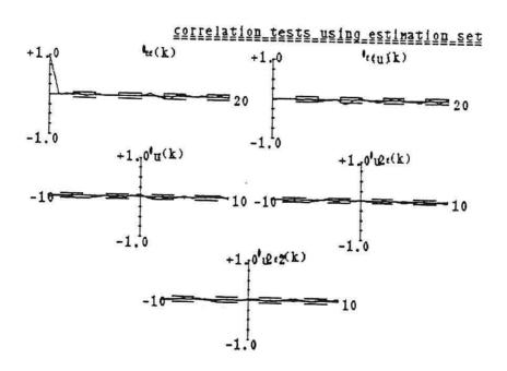
Figure 5.4 Model validation for the dynamic system with dead zone & saturation
