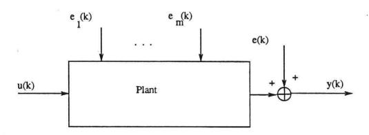
(b) Current noise at the input and output
