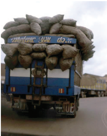
Figure 4.2 – Overloaded vehicles are often responsible for structural damage to the road structure (photo courtesy: P. H. Bentall).
