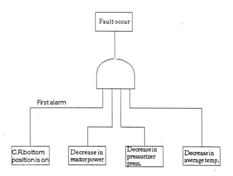
Figure 2: Fault tree for the rod drop fault
