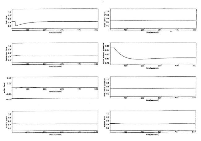
fig. 6: The boiler response to drum steam pressure demand change with two Pl regulator
