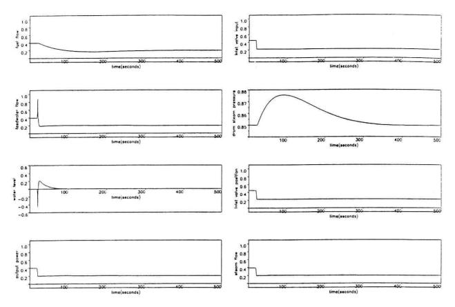
fig. 5: The boiler response to output power demand change with two PI regulator
