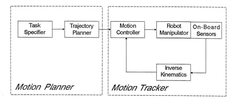
Figure (1): The Robot Integrated System
