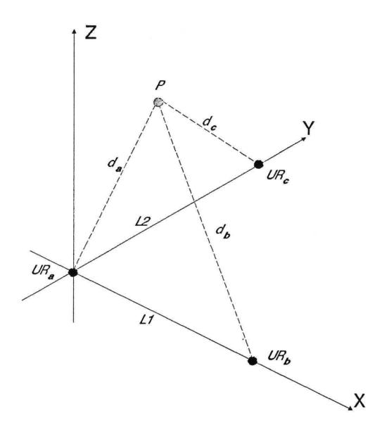
Figure (3): 3-D Position Measurement
