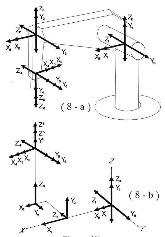
Figure (8): Frames Assignment for a PUMA-like Arm
