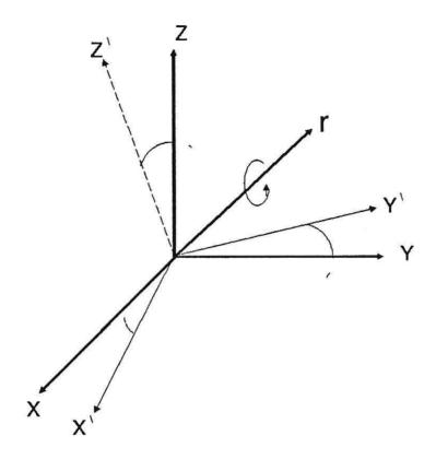
Figure (12): Rotation About an Arbitrary-Axis
