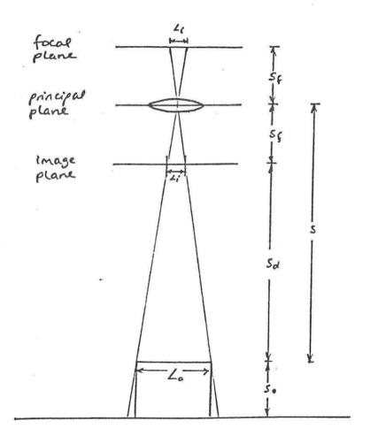
Figure 10. Perspective projection of the object due to the camera
