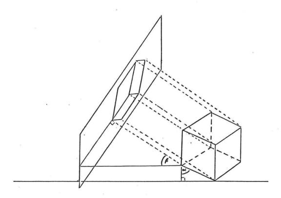
Figure 1. Diagram illustrating the angle of viewing  $\beta$  and the angle of orientation  $\alpha$  with respect to the plane onto which the object is to be projected.
