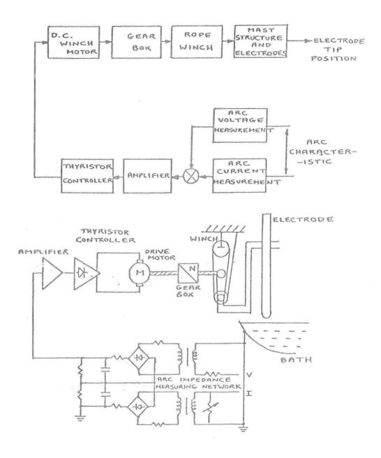
A direct-haul d.c. motor driven electrode position controller
