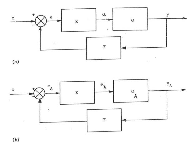
Fig. 1 (a) Real and (b) Approxmating Feedback Systems
