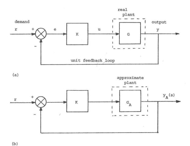
Fig. 1. Real (a) and Approximating (b) Feedback Control Schemes
