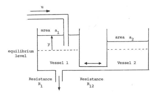
Fig. 5. Liquid Level System
