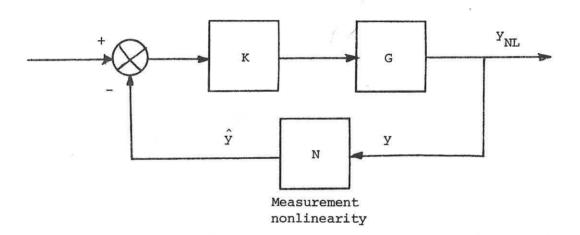
Fig. 10. Multivariable Feedback System with Measurement Nonlinearity
