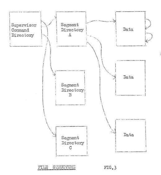
Typically a user will require some 10 - 15 K words of storage for this purpose 4 and since on the CONPAC disc file there are approximately 100 K words of unused storage the system should be capable of handling 8 - 10 users. A user will be able during the 'login' procedure to overlay the contents of his own data files into the working files .
