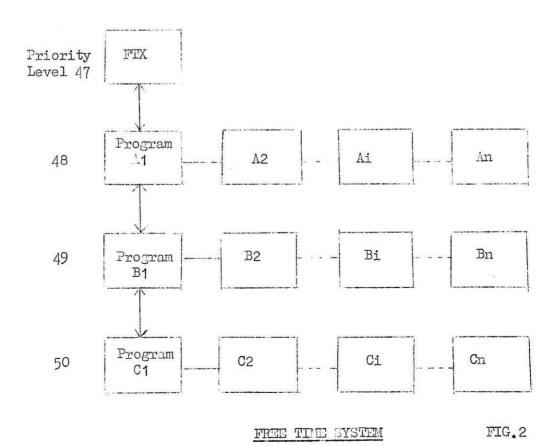
any other free time program Ai(i=2,n), Bi(i=1,n), Ci(i=1n) or can run any free time program at priority level 49. Similarly any program running at priority level 49 can replace itself at level 49 or can run a program at level 50. Programs running at level 50 can only replace themselves. All programs on termination return control to the program running at the next highest level.
