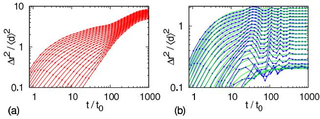
FIG. 4: (*Color online*) Mean squared displacement  $\Delta r^2(t_w + t, t_w)$  for single runs at (a)  $\phi = 0.8 < \phi_J$  and (b)  $\phi = 0.88 > \phi_J$ . In both cases, lines from top to bottom correspond to geometrically increasing  $t_w$  in the range  $0.4 < t_w/t_0 < 40$ . In (b) the smooth green lines are smoothing fits (see text).
