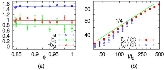
FIG. 5: (*Color online*) (a) Transport and aging exponents versus density. Smooth lines are the average over all  $\phi$ . (b) Characteristic cluster size  $\xi_c$  and velocity correlation length  $\xi_v$  at late times for  $\phi = 0.7$ .
